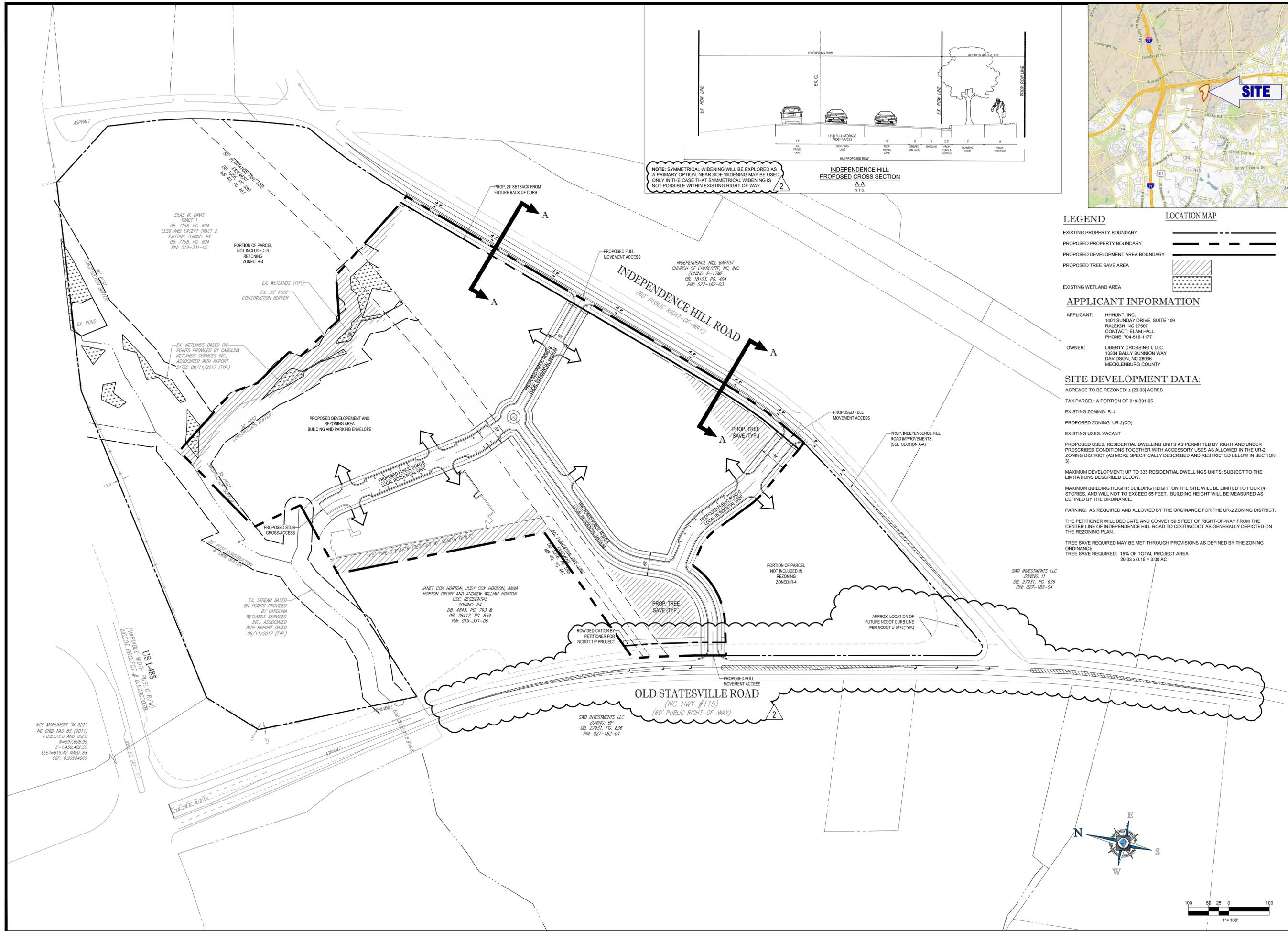
NOTE: SYMMETRICAL WIDENING WILL BE EXPLORED AS A PRIMARY OPTION. NEAR SIDE WIDENING MAY BE USED ONLY IN THE CASE THAT SYMMETRICAL WIDENING IS NOT POSSIBLE WITHIN EXISTING RIGHT-OF-WAY.
