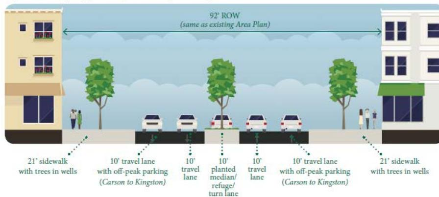
Figure 7a: South Tryon Segment 1 Proposed Section (Long term)
