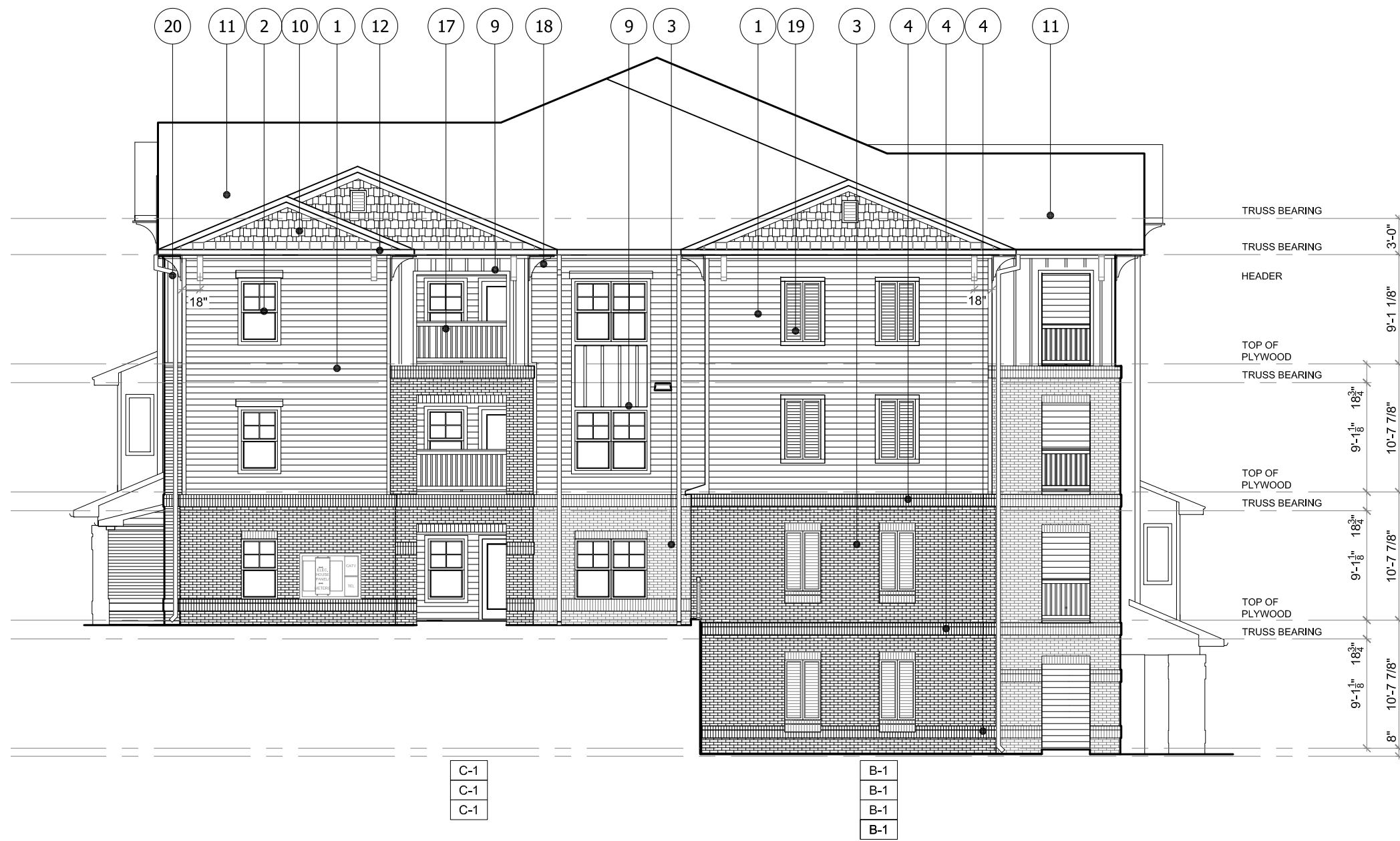
2 TYPE 4 (BLDGs - 3, 4, 5 & 7) - RIGHT ELEVATION A5-4 1/32"=1'-0"
