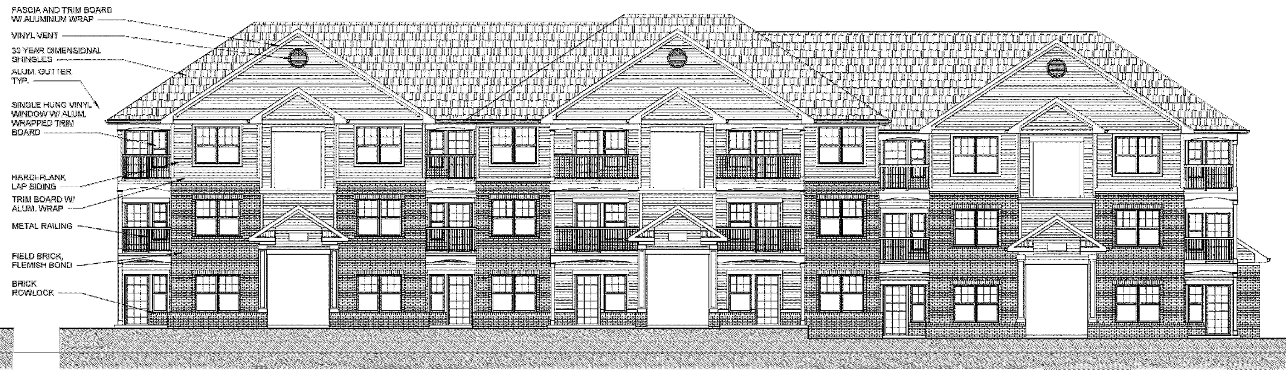
1 12B6C FRONT ELEVATION 1/8" = 1'-0"
