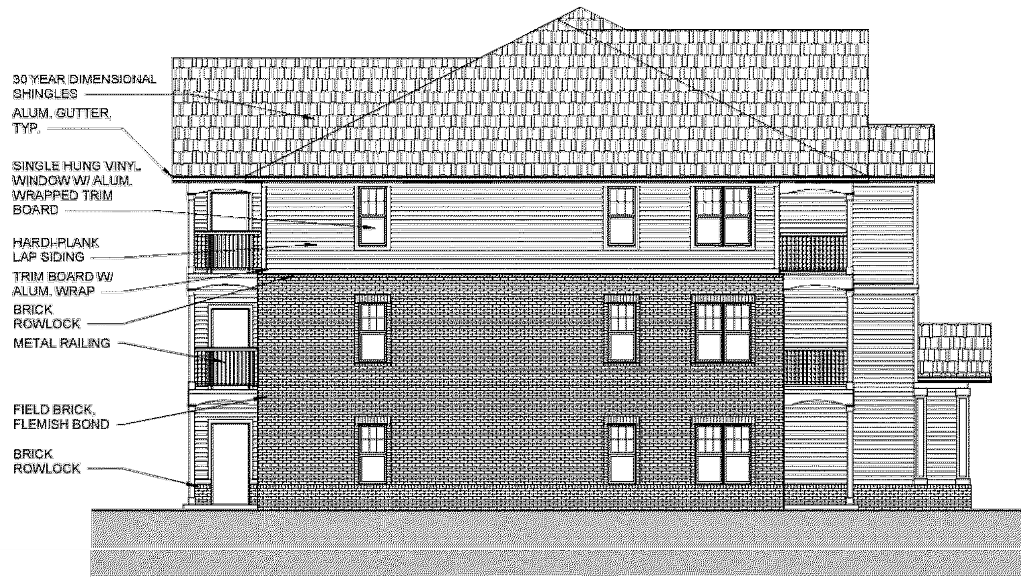
2 12B6C LEFT ELEVATION 1/8" = 1'-0"
