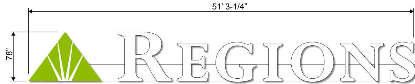
RFC.REG-IL78MWL-RW - 78”H ILLUMINATED WHITE MODIFIED LINEAR RACEWAY CHANNEL LETTERS SCALE: 1/8" = 1' 0"
