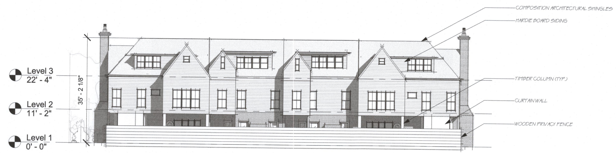
1 FRONT UNIT REAR ELEVATION 1/16" = 1'-0"
