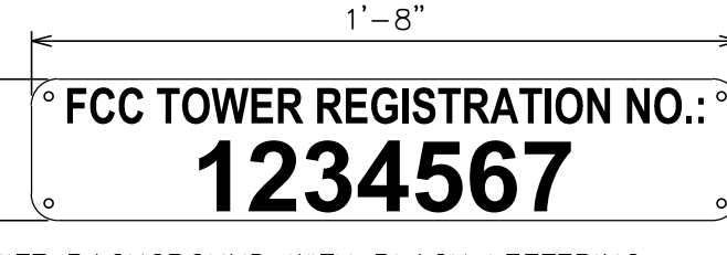
⑥ WHITE BACKGROUND WITH BLACK LETTERING QUANTITY: (2) TO BE MOUNTED ON: COMPOUND ACCESS GATE ACCESS DRIVE GATE (SEE NOTE 4)
