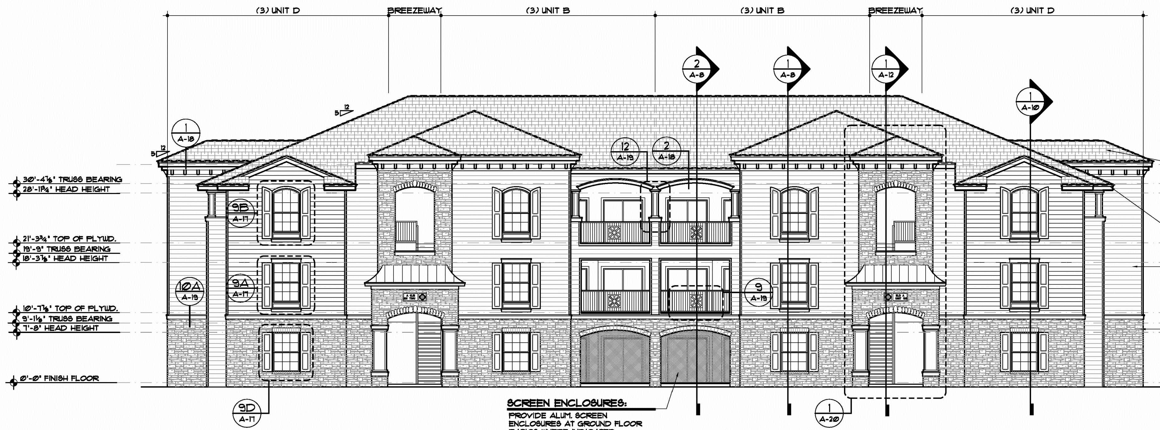
1 BUILDING TYPE SIX - FRONT / REAR ELEVATION
