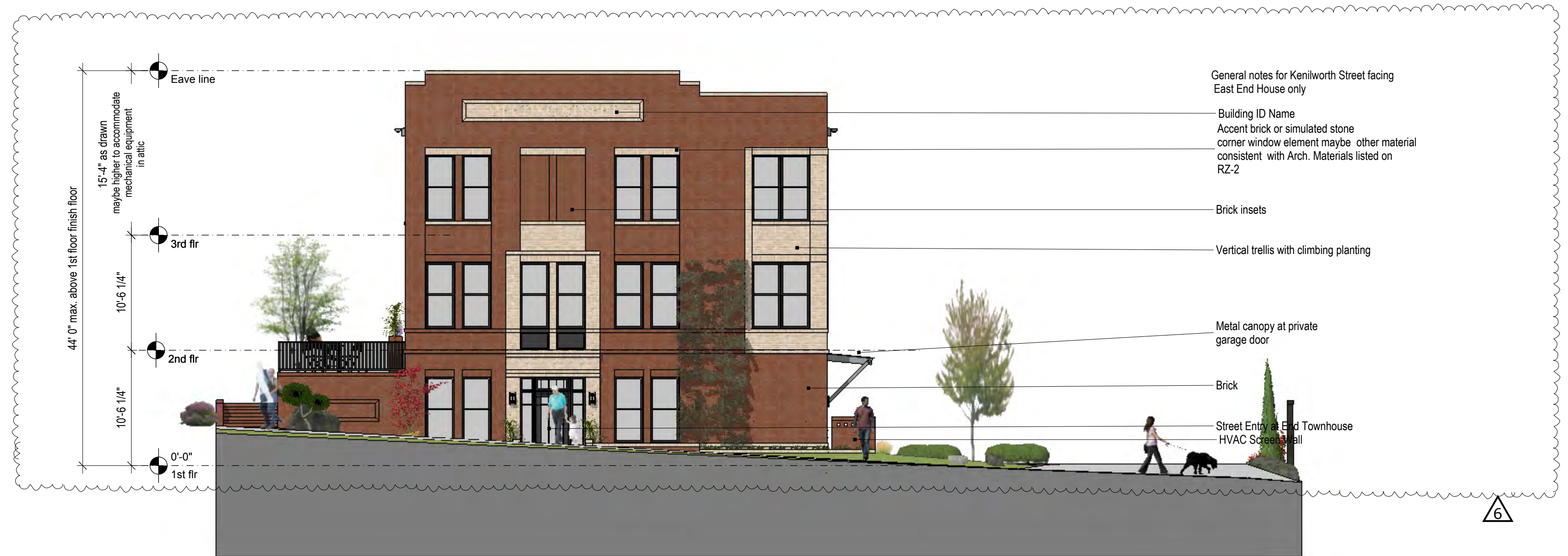
C :: East Elevation (Kenilworth Avenue) RZ3 scale: 1/8"=1' 0"
