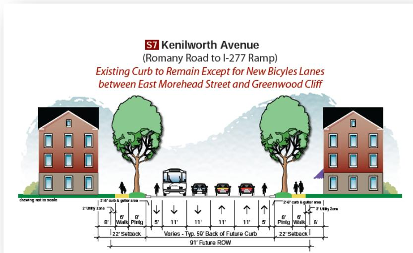
**Figure 1: Recommended Kenilworth Street Cross Section**
