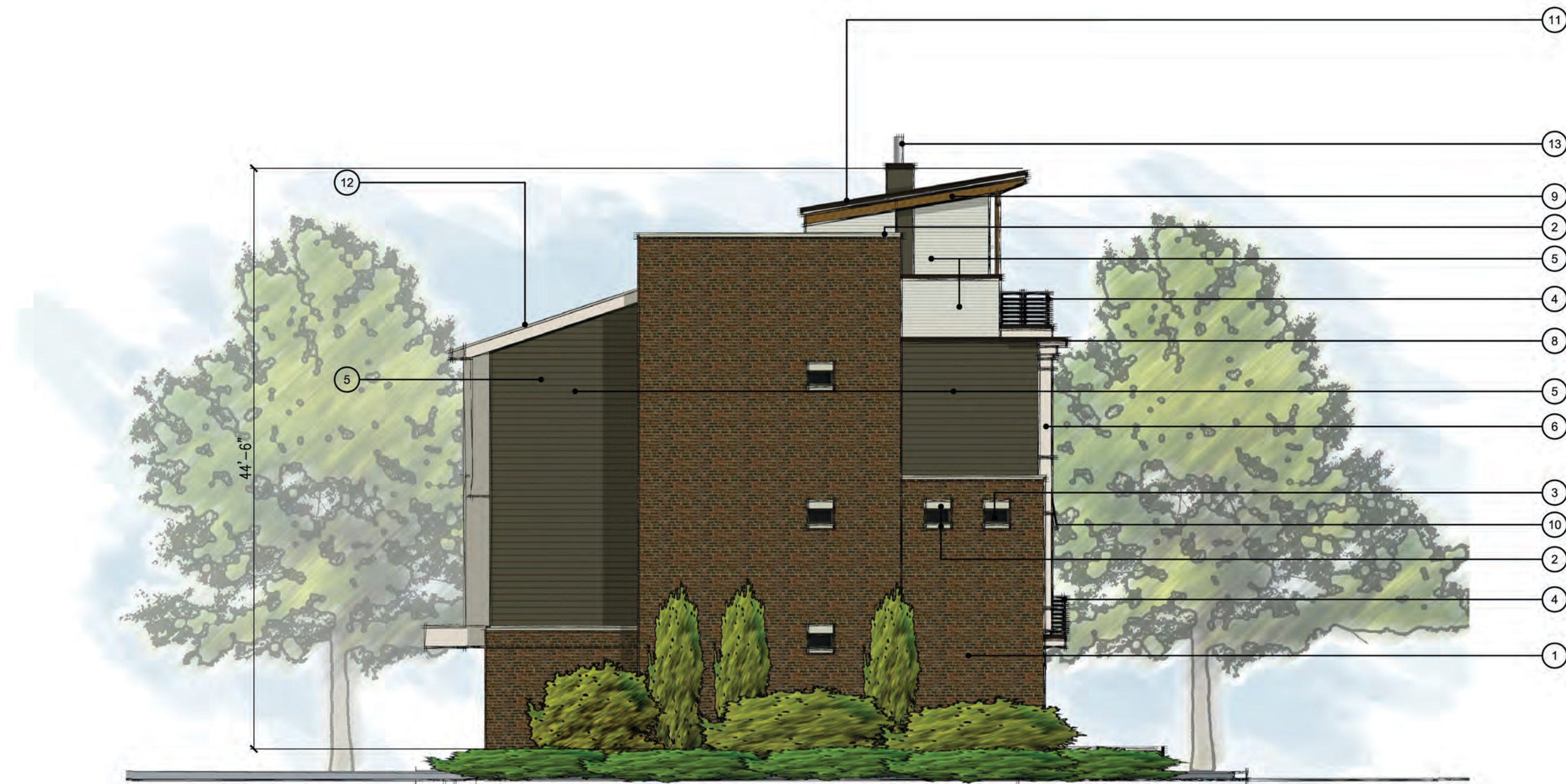
2 TYPICAL SIDE ELEVATION - PHASE 1 & PHASE 2 Scale | 1/8" = 1'-0"
