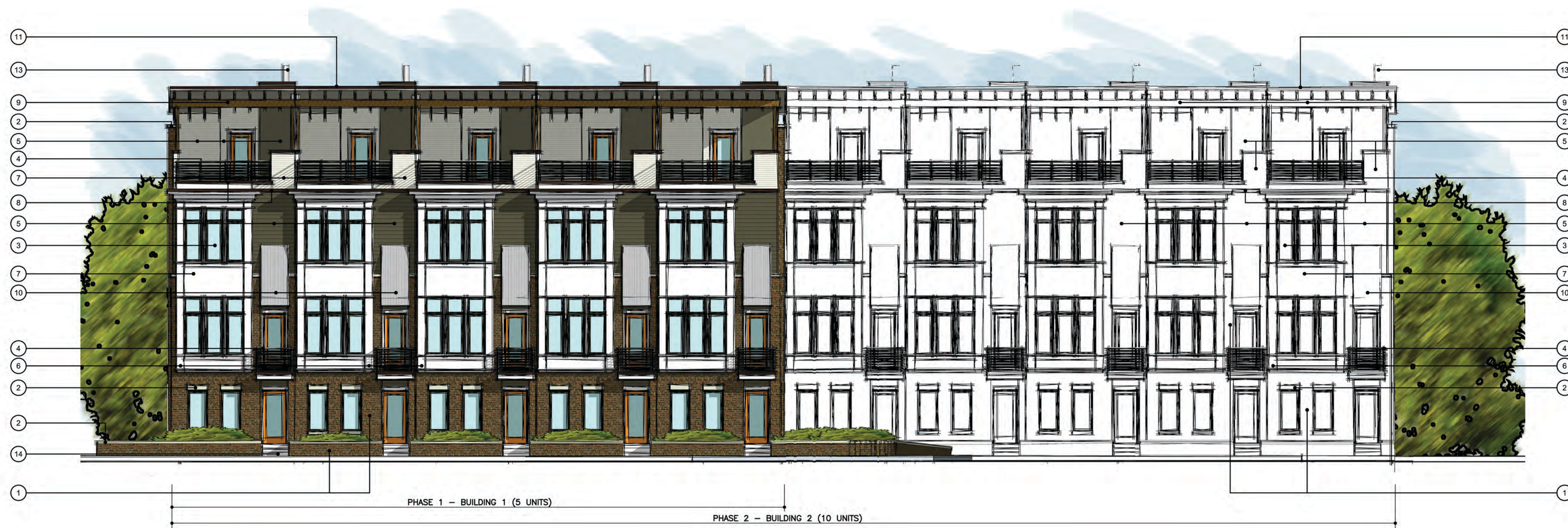
1 FRONT 35th & YADKIN STREET ELEVATIONS Scale | 1/8" = 1'-0"
