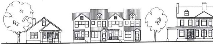
New construction can make use of architectural elements found on adjacent buildings, such as gables and porches, to create appropriate mass by breaking up long facades.
