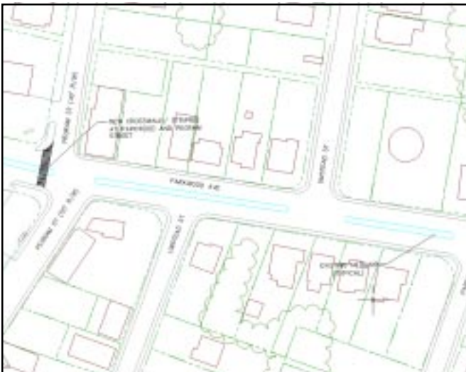
PARKWOOD / PEGRAM STREET PEDESTRIAN CROSSING
