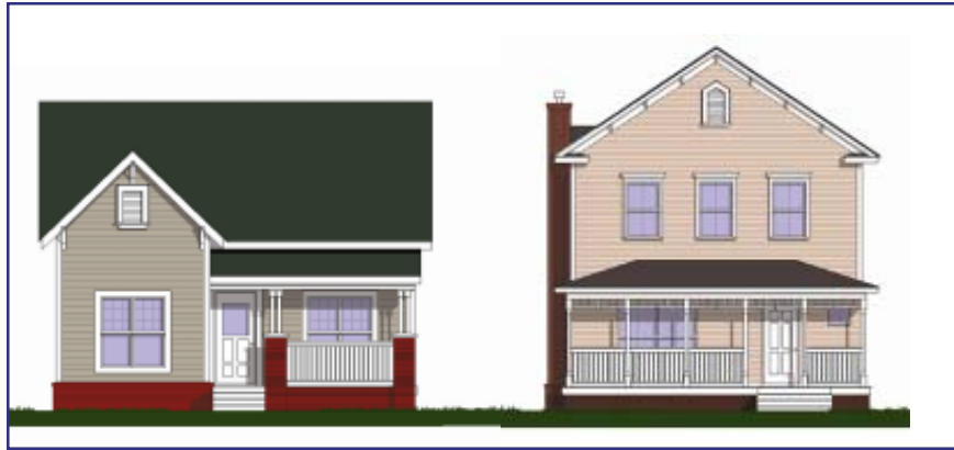
Roofs of new infill housing units should be of simple form and consistent with existing historic housing. Roofs should have a pitch of at least 8/12 and an overhang of at least 12" wide.
