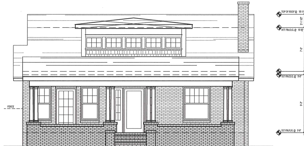
2 EXISTING FRONT ELEVATION 1/4" = 1'-0"
