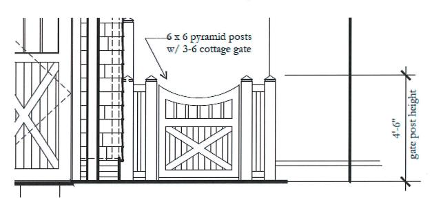
Fence design for left and right sides of carriage house.
