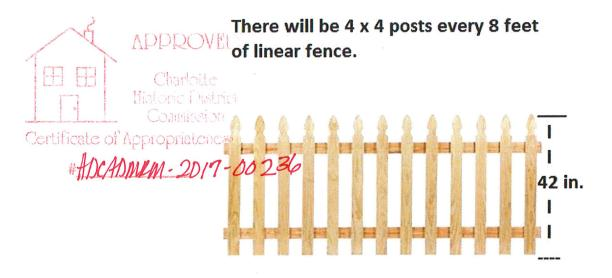
In red, is where the proposed fence will be added to the property with the dimensions of each section.
