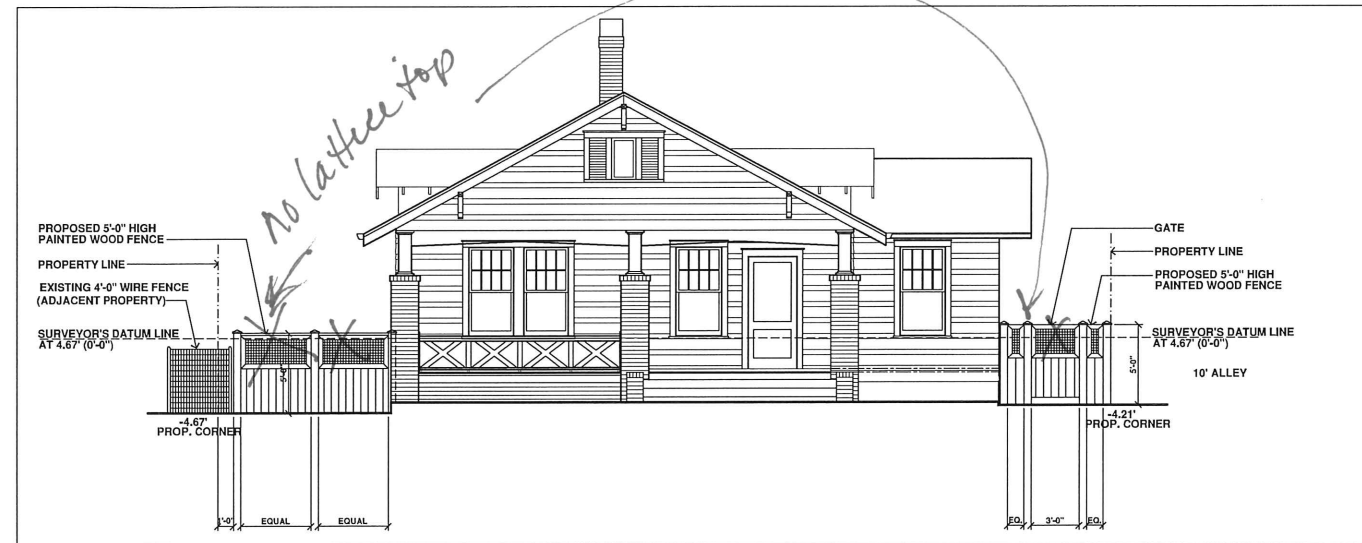
B FENCE ELEVATION FROM PARK ROAD SCALE: 3/16" = 1'-0"
