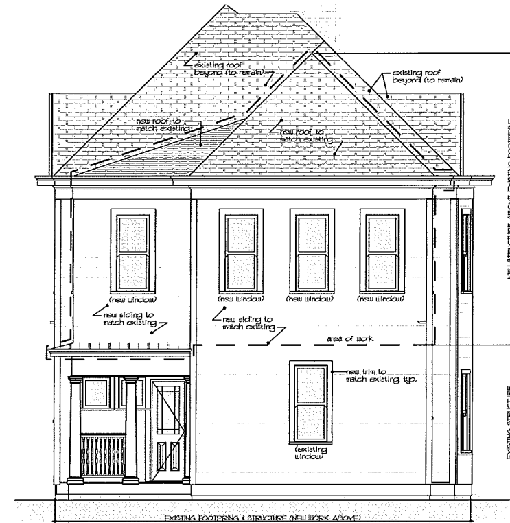
3 A2.2 PROPOSED REAR ELEVATION SCALE: 1/4" = 1'-0"
