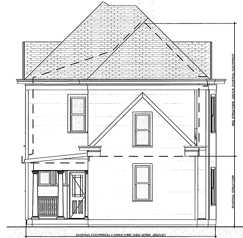
1 A2.2 EXISTING REAR ELEVATION SCALE: 1/4" = 1'-0"
