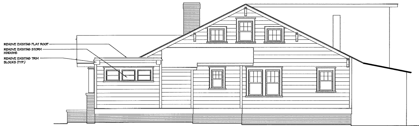
Right Side Elevation - EXISTING
