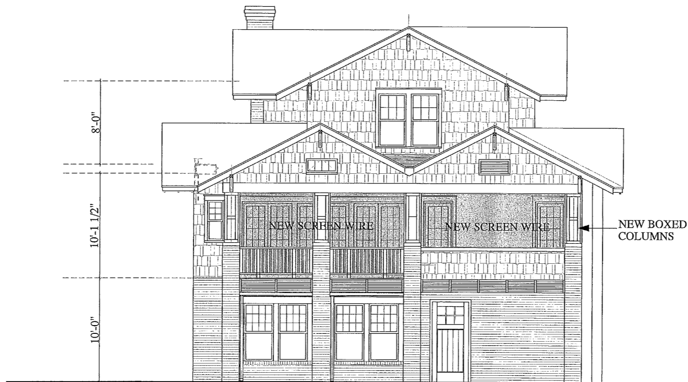
2 NEW NORTH ELEVATION (REAR) A4 1/4" = 1'-0"
