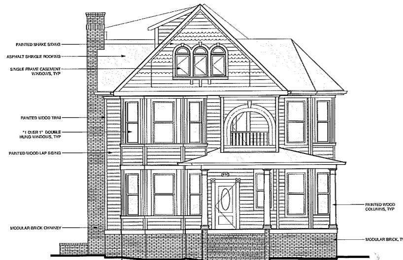
C1 Existing North Elevation (Front) Scale: 1/4" = 1'-0"
