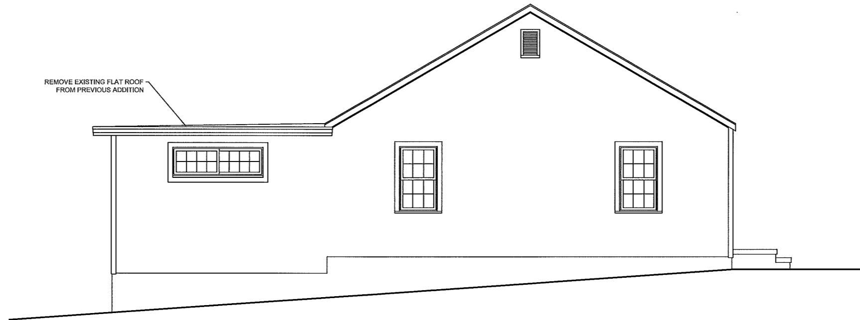
EXISTING LEFT SIDE ELEVATION \frac{1}{4}'' = 1'-0''
