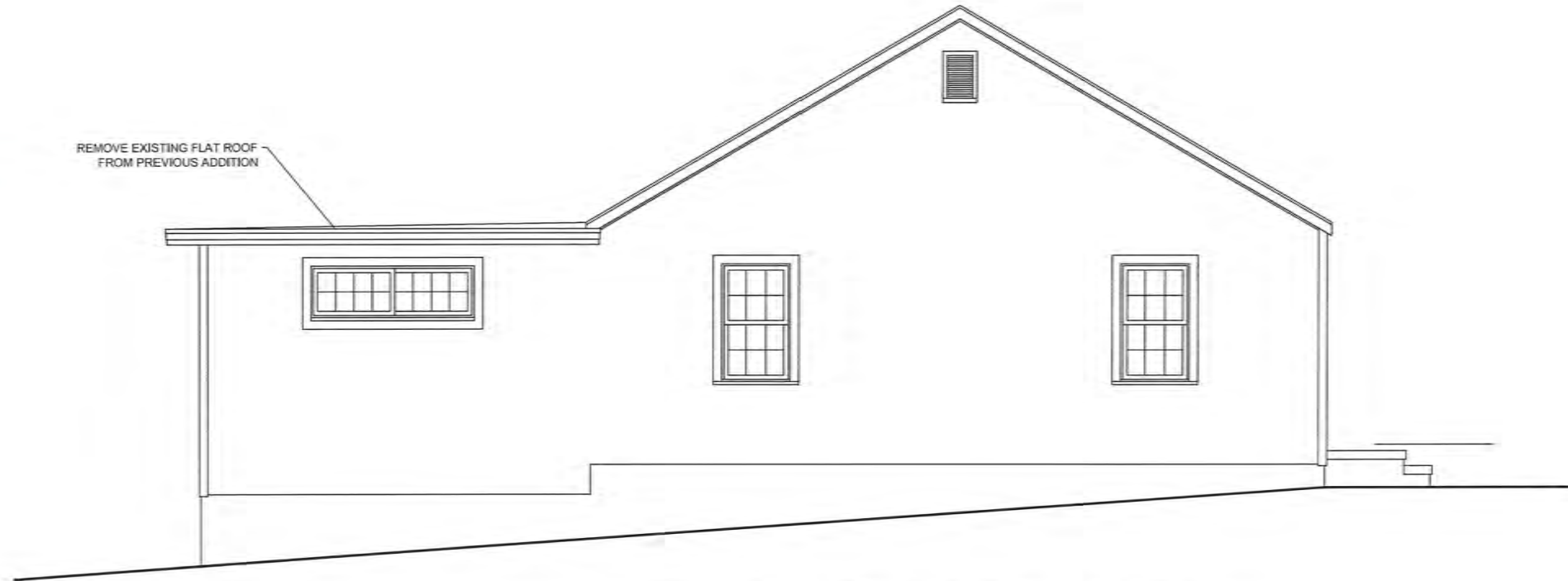
EXISTING LEFT SIDE ELEVATION 1/4" = 1'-0"
