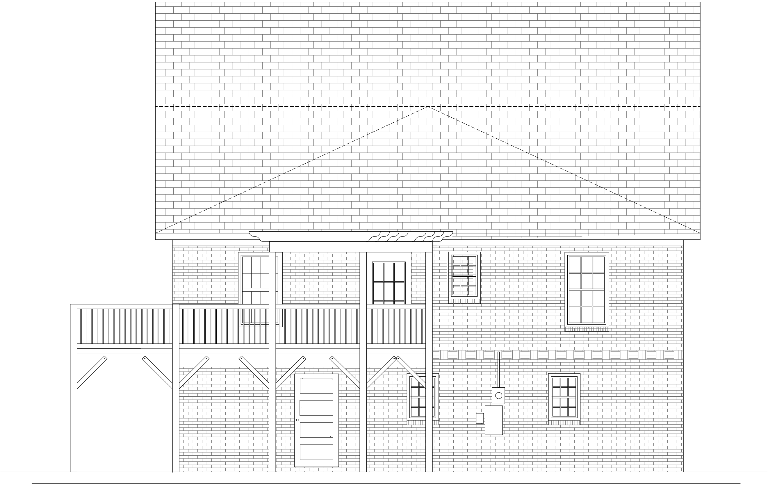
REAR ELEVATION SCALE: 1/4" = 1'-0"
