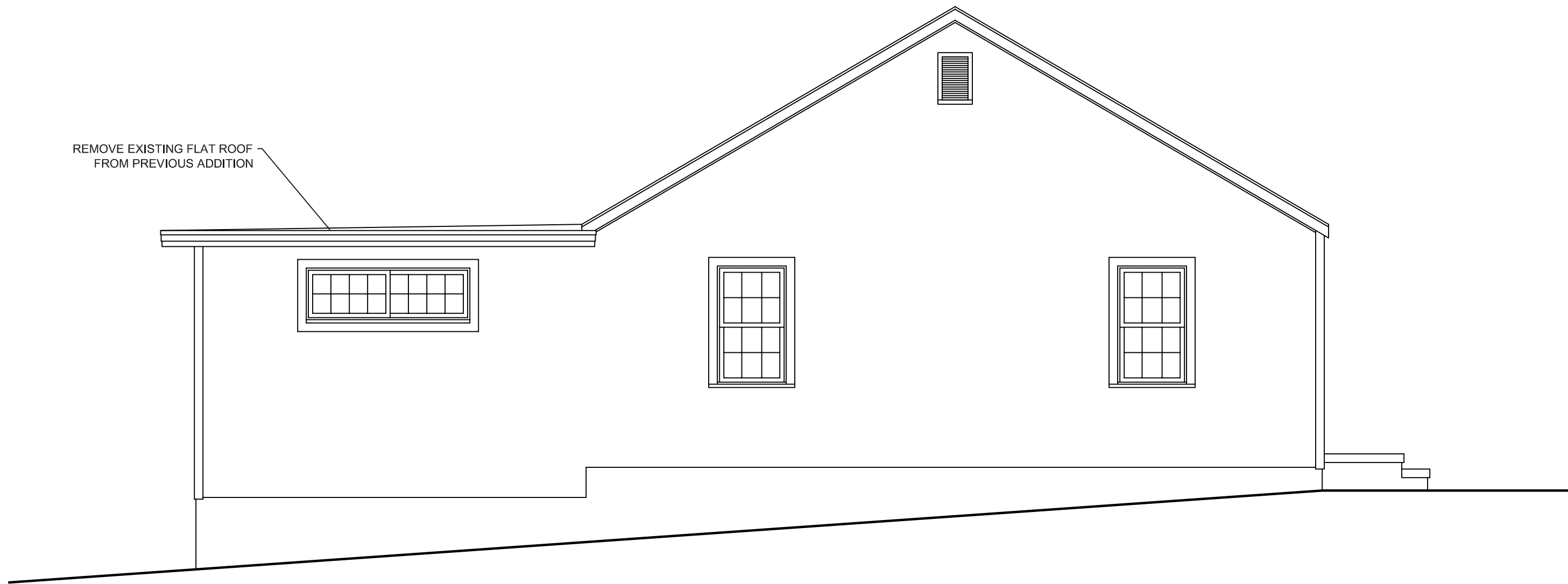
EXISTING LEFT SIDE ELEVATION 1/4" = 1'-0"
