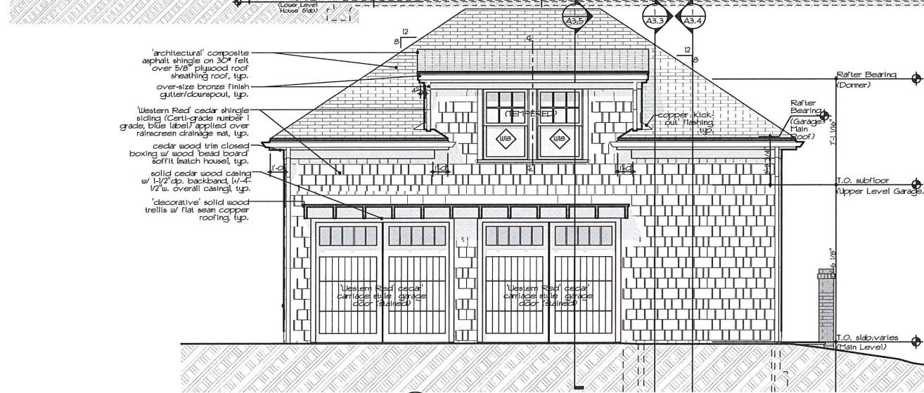
5 Rear Elevation - Garage SCALE: 1/4" = 1'-0"
