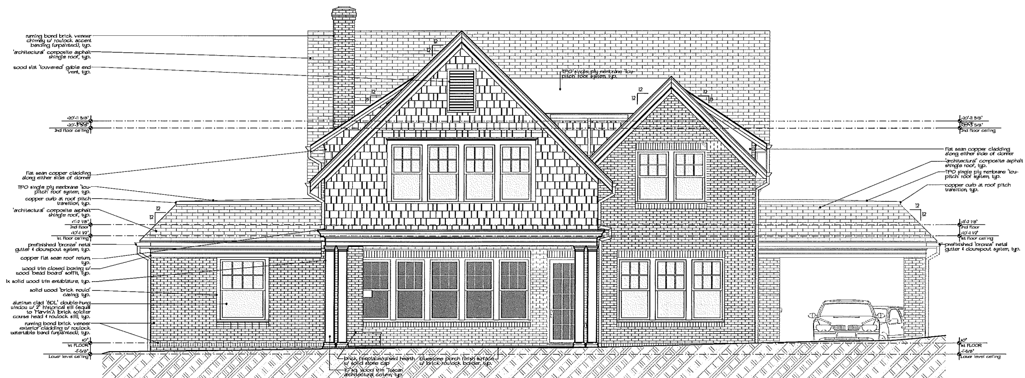
1 Rear Elevation A2.2 SCALE: 1/4" = 1'-0"
