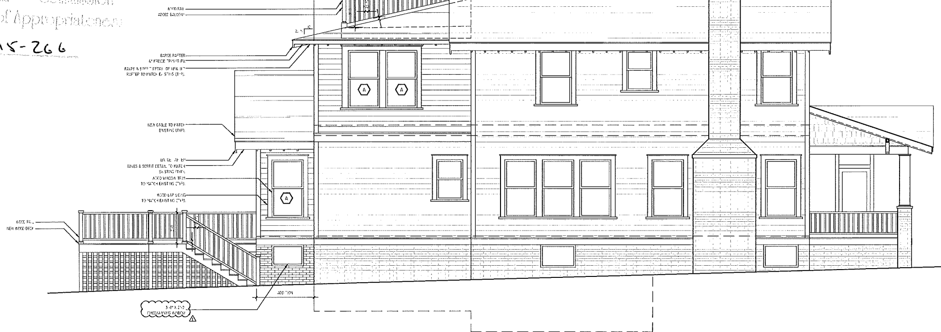
② PROPOSED LEFT SIDE ELEVATION (WINTHROP FACING) 1/4" = 1'-0"
