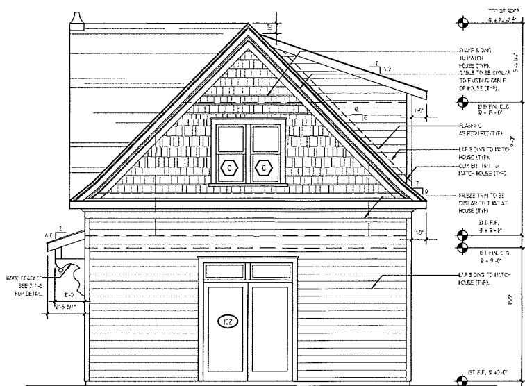
② RIGHT SIDE ELEVATION (ALLEY FACING) 1/4" = 1'-0"
