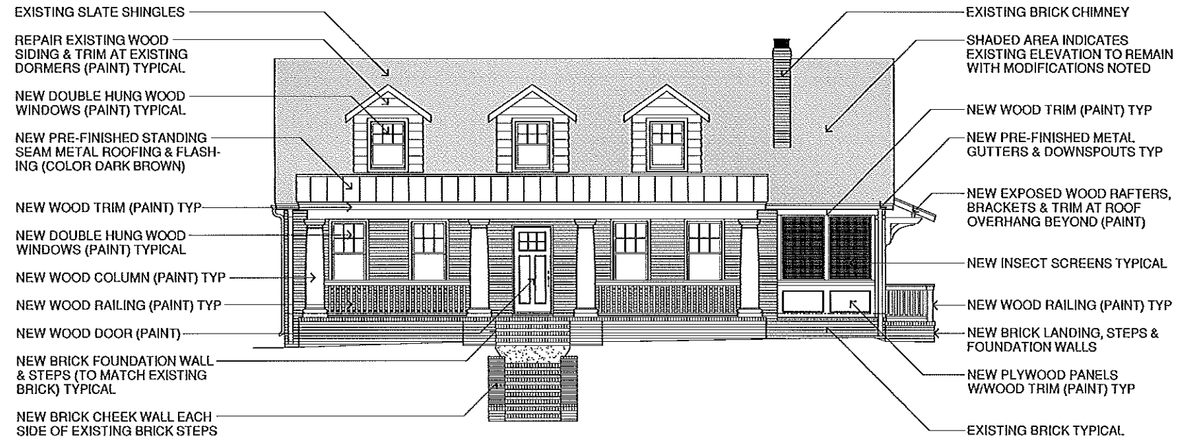
B PROPOSED FRONT ELEVATION SCALE: 1/4" = 1'-0"
