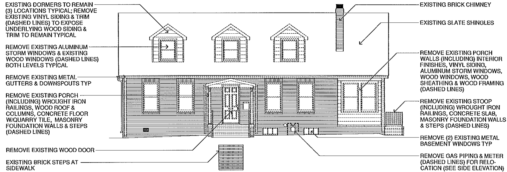
A EXISTING / DEMO FRONT ELEVATION SCALE: 1/4" = 1'-0"
