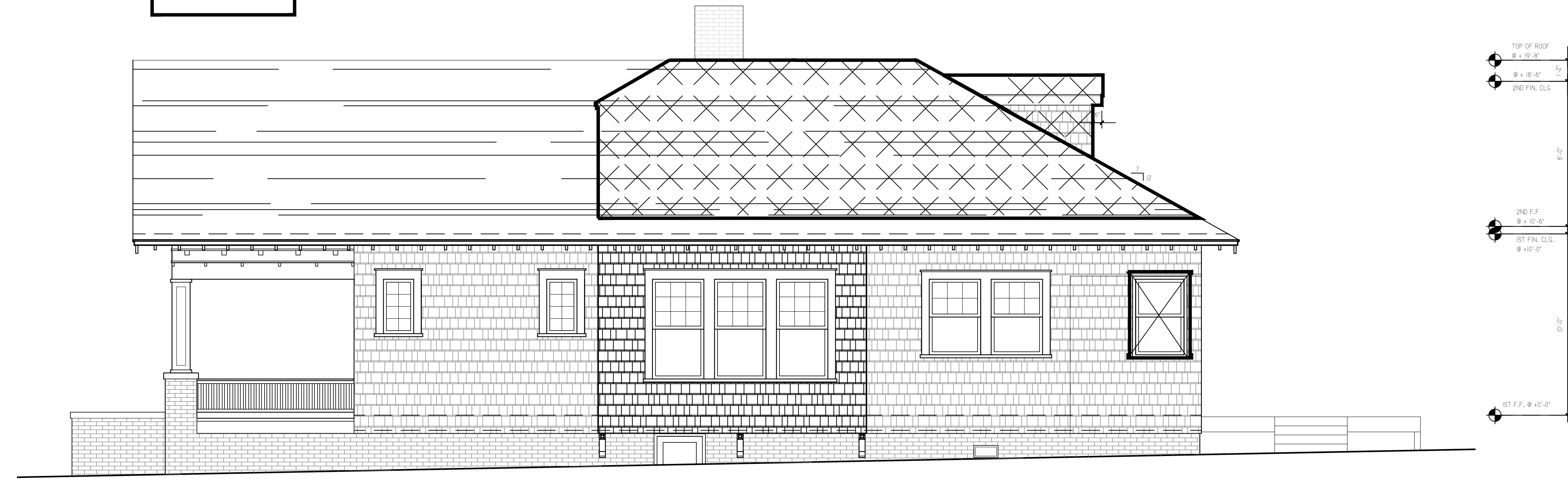
② EXISTING RIGHT ELEVATION 1/4" = 1'-0"
