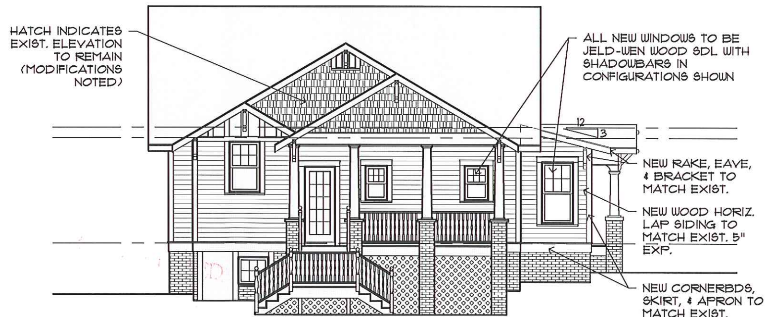
2 REAR ELEVATION (SOUTH) - PROPOSED A2.2 SCALE: 1/8"=1'-0"
