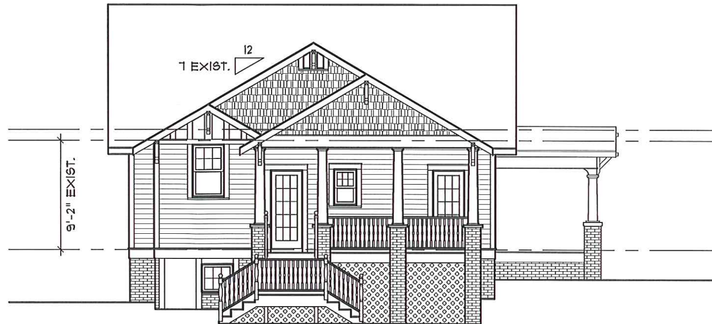
1 REAR ELEVATION (SOUTH) - EXISTING A2.2 SCALE: 1/8"=1'-0"
