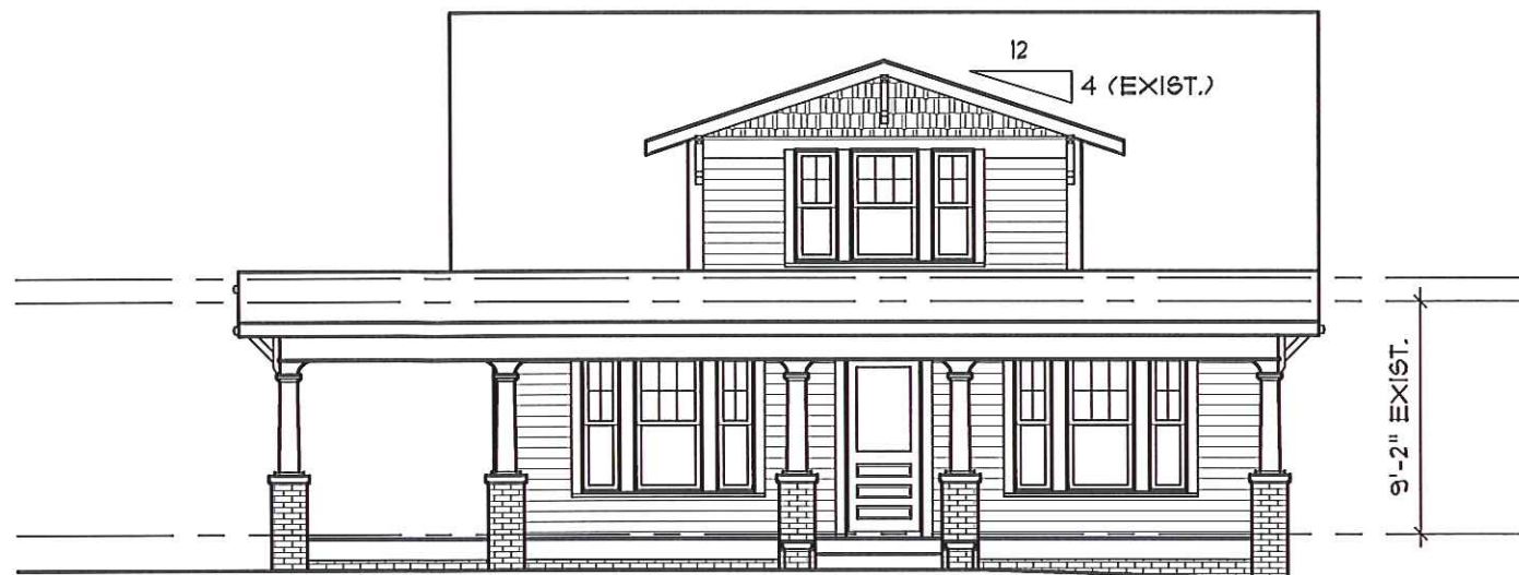
1 THE PLAZA ELEVATION (WEST) - EXISTING A2.0 SCALE: 1/8"=1'-0"
