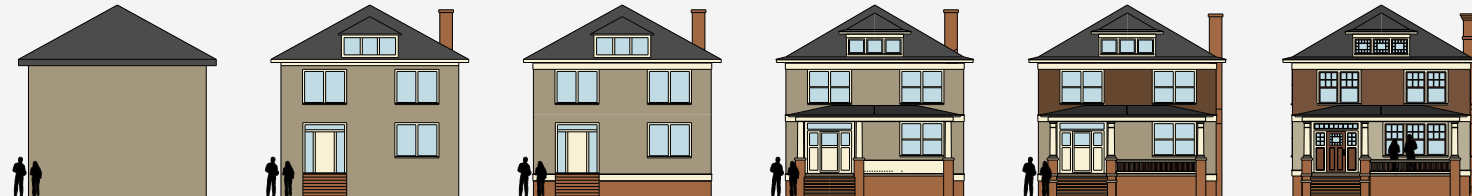
This illustrates how (from left to right) features such as windows and doors, foundation articulation, porches, materials and window detail create scale that relates a building to the human scale.
