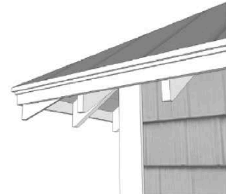
Craftsman styled trim details may include corner boards and exposed rafter ends.
