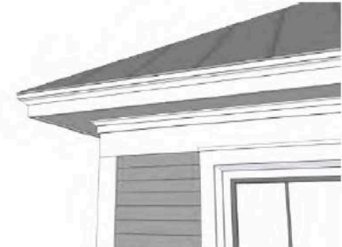
On many different styles flat boards with simple trim define exterior elements such as eaves, corners and windows.
