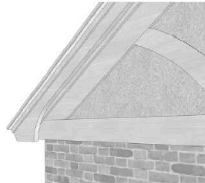
Half-timber framing on Tudor Revival houses is actually just composed of decorative trim boards.
